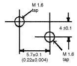
**Note:** Unless otherwise specified, a tolerance of  $\pm$  0.2 mm applies to all dimensions.
